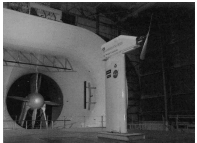
Fig. 3 Propeller test stand installed in LFST.
