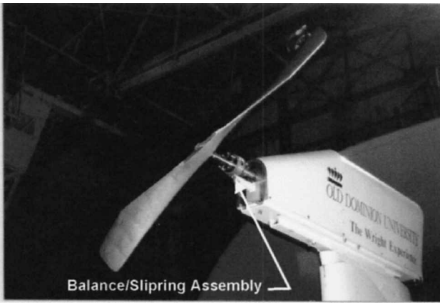
Fig. 4 Test propeller installation showing balance and slirping assembly.
